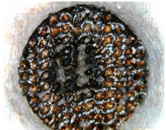
Fig. 1 Ag/Ni contact processed by electron beam to create a highly structured surface (Diameter 2.5mm).
